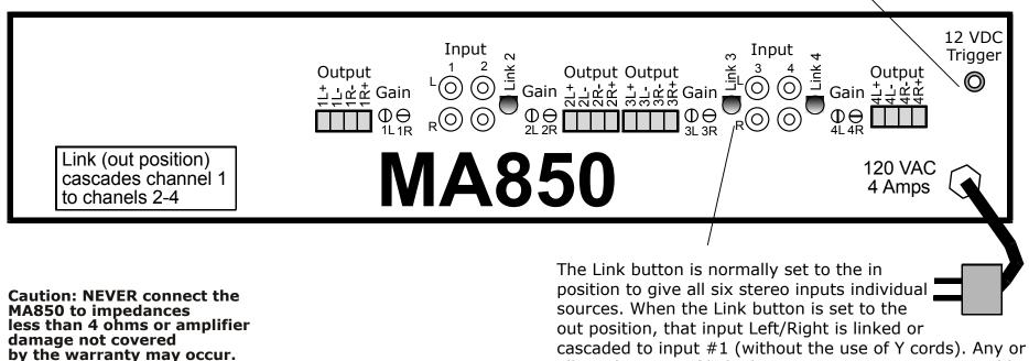
all combination of linked inputs 2 to inputs 6 are possible. When all inputs are linked to input 1 the input impedance is about 4000 ohms.
